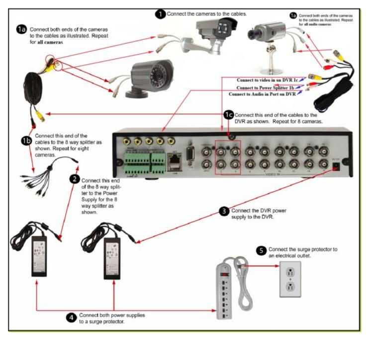
Please note that it is STRONGLY recommended to use a surge protector that is UL-1449 rated. Look for a clamping voltage of 330 or lower, a Joule rating of at least 400 and a response time of 10 nanoseconds or less.
